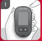
Press and release (power/set button) to (power/set button) to turn the meter on. The flashing test strip symbol appears on the display.
