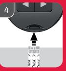
Insert the test strip into the meter in the direction of the arrows. The meter turns on and beeps.
