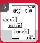
Use  $\triangleleft$  or  $\triangleright$  to adjust the hour. Press and release  $\bigcirc$  to advance through the hour, minutes, day, month and year, adjusting each flashing setting as needed with  $\triangleleft$  or  $\triangleright$ .
