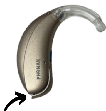
Open Battery Door Turned OFF
