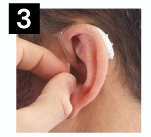
Tuck the retention wire into the bowl of the ear to secure the device
